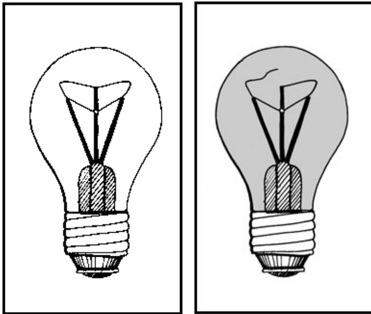
*Which light bulb has a closed circuit?*
