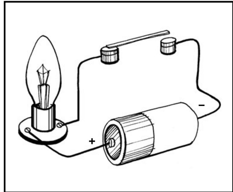
Another way to demonstrate a circuit is to look at a light bulb. A light bulb has a tiny wire, or filament, in it. Electricity enters the light bulb and passes through the wire. The wire heats up and glows creating light. After a while, the wire wears out and breaks. The electric circuit becomes open and electrons can no longer flow through the wire. You have to buy a new light bulb with an unbroken filament.
