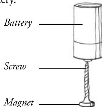
4. Press and hold one end of the wire to the top of the battery.
